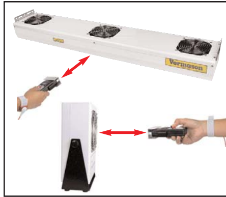
Figure 3. Auditing ionisation equipment with the Digital Static Field Meter and Conductive Plate
