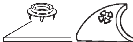
Figure 9. Installing push and clinch mat grounding snap.
