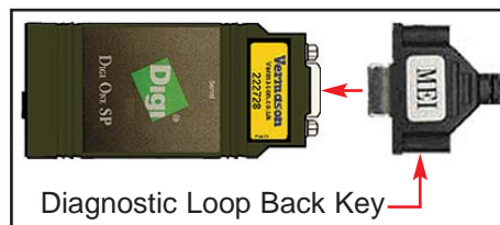
Figure 3. Connecting the Diagnostic Loop Back Key
