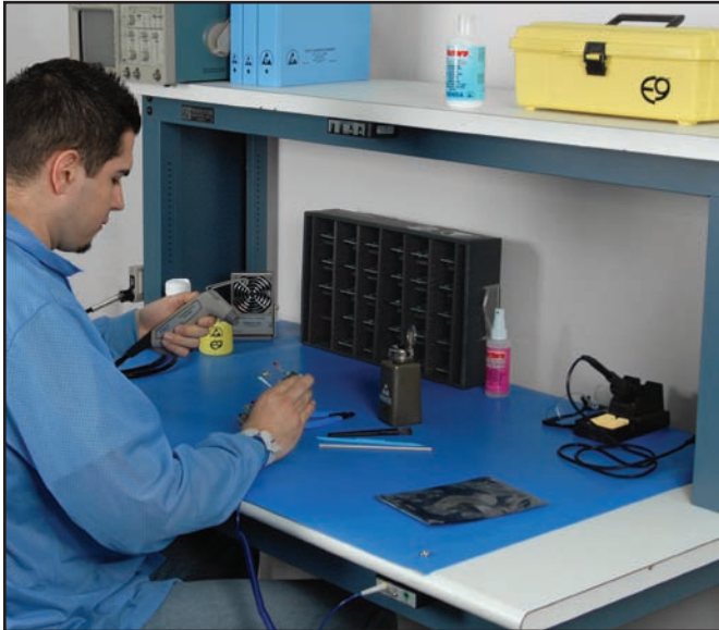
Figure 8: Using the Chargebuster Ion Gun
